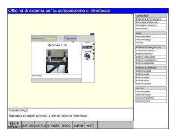
Fig. 15. Using W-Client system workshop, a d-expert is creating the application workshop shown in Fig. 12. The button "diagnostica" (diagnostic) is being located on the operative button panel.
