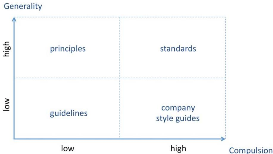
Fig. 6. Classification of design recommendations (adapted from [16])
